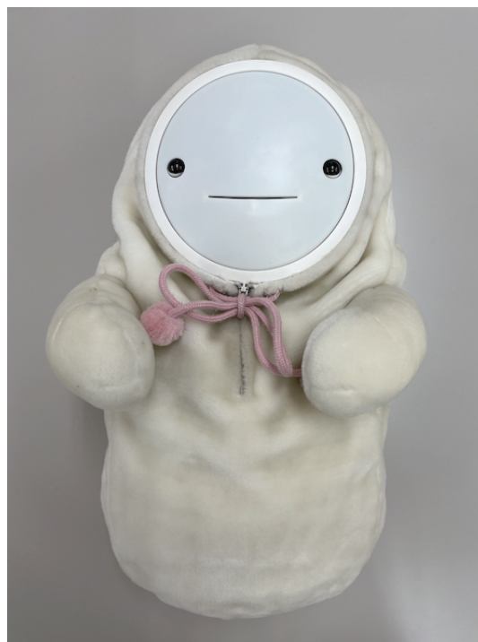
Figure 1 “Smibi®”, a healing baby companion robot. This companion robot was produced by the Togo Seisakusyo Corporation. The main body weighs 1.2 kg and has a width, depth, and height of 200 mm, 190 mm, and 440 mm, respectively. The power source is a lithium-ion battery that can be used for approximately 10 hours without charging. It uses a dedicated adapter for charging. The robot expresses emotions in 500 different ways, and its responses vary depending on how the user interacts with it.
